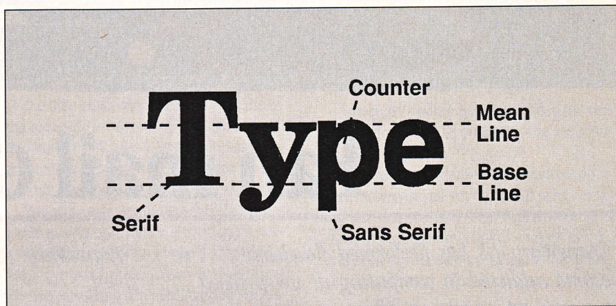
This "type" diagram shows the difference between serif and sans serif letters. Serifs are any of the short lines that emerge from — and at an angle to — the upper and lower ends of a letter. Fonts with serifs are easier to read.
